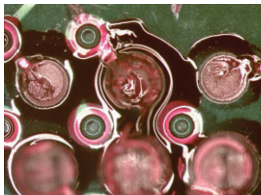
Figure 17B Dye & Pry Image PCB Side (pin A26, board 17159)
