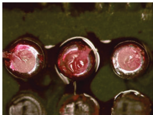
Figure 17A Dye & Pry Image BGA Side (pin A26, board 17159)
